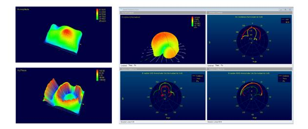
With the Circular Polarization (CP) option, the RFS calculates the right and left hand circularly polarized patterns and displays axial ratio patterns. RFS can be integrated into virtually any automated test bed and production line by using DLL programming.
